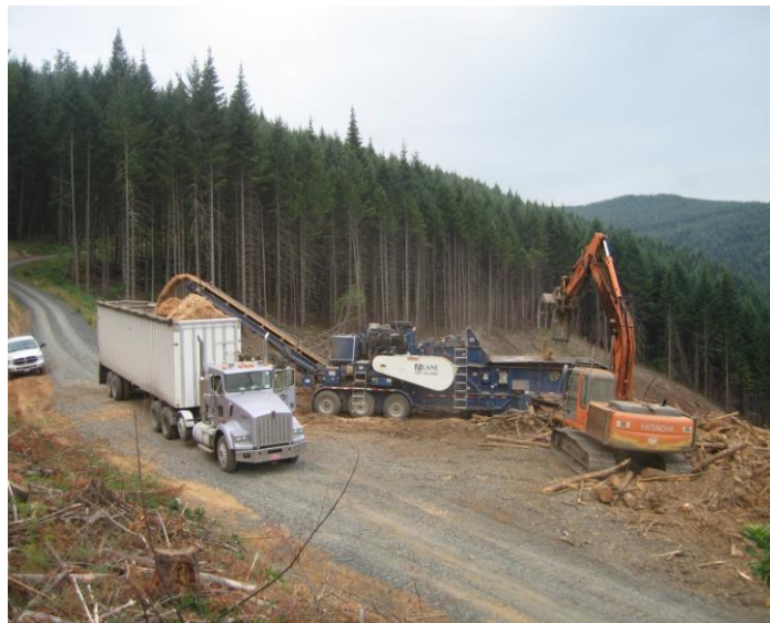
Figure 1. This image shows the traditional conveyor belt distribution method. Reference
