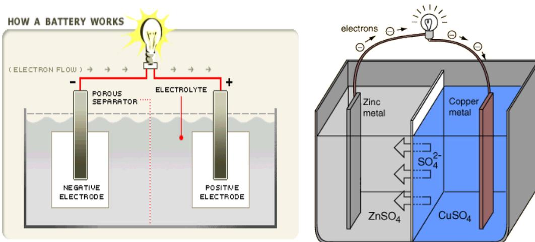
Figure 1. Electron flow in batteries
