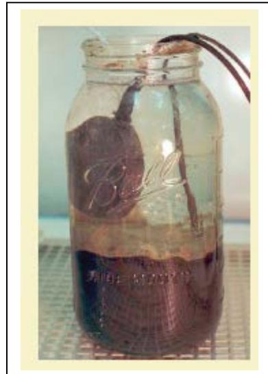
\*One example of a mud bacteria fuel cell is the picture above; this was created with graphite electrodes in a mason jar.
