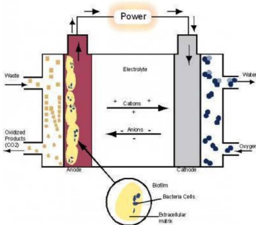
Figure 1. A simple microbial fuel cell. [Reference](#)
